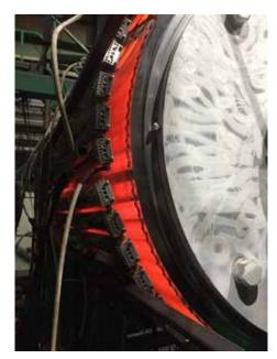
Infrared panels enable to heat quickly rotating metal objects without contact
